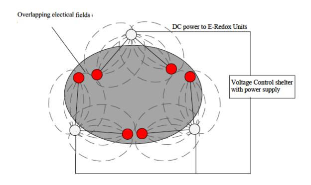
Figure 5. E-Redox<sup>®</sup> system layout for source area treatment
