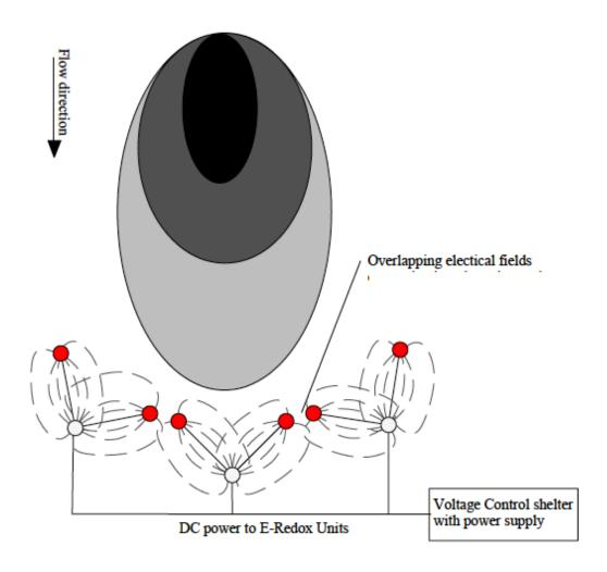
Figure 4. E-Redox<sup>®</sup> system layout for treatment of a contaminant plume
